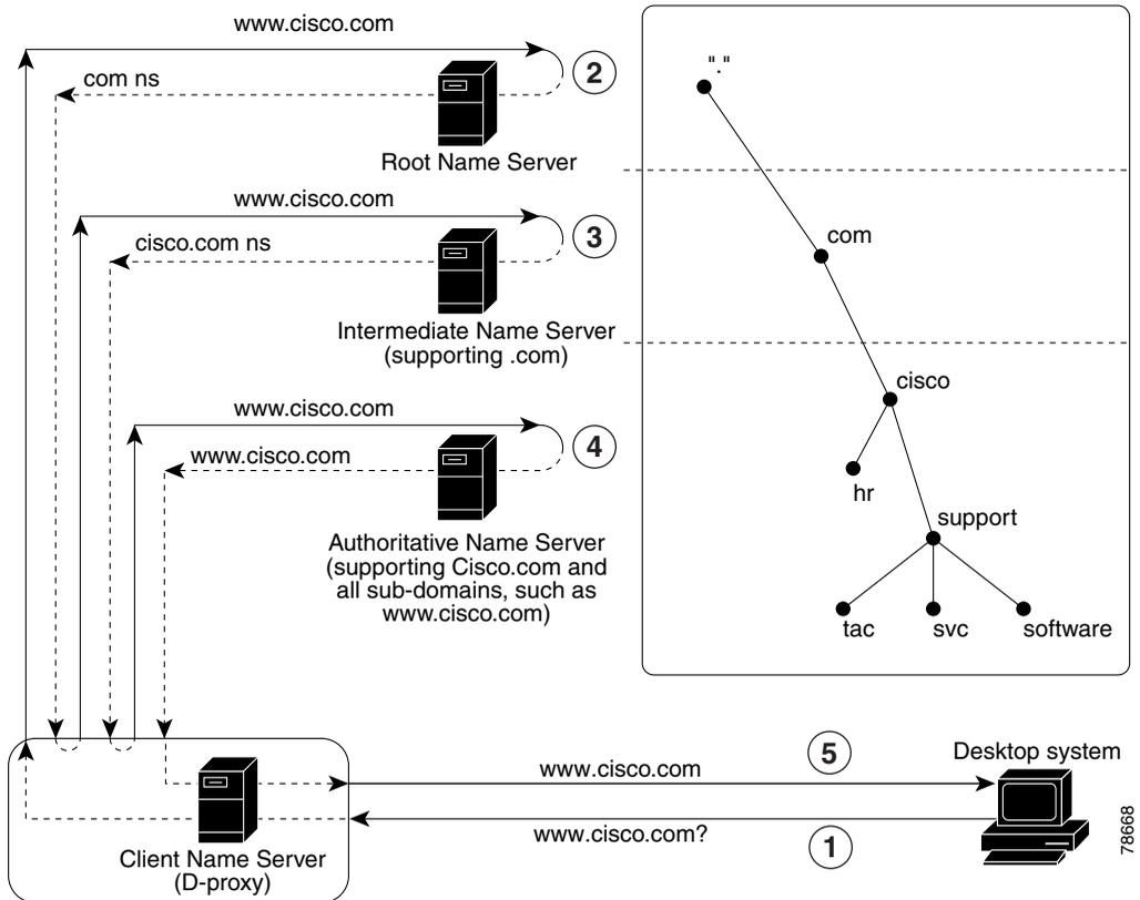
1. The resolver (client) sends a query for `www.cisco.com` to the local client name server (D-proxy).
